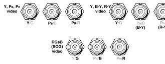
Figure 4 — Input connections
